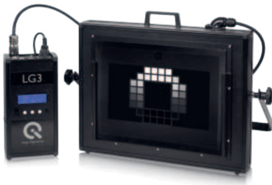
LG3 with OECF test chart TE269C
