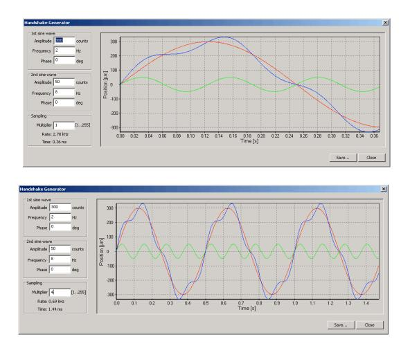
The amplitude is given in "counts" which is the metric of the positioning sensors. One count corresponds to one micrometer. Please note that the amplitude here denotes the displcement between the sensor and magnetic tape, the corresponding total travel of the voice coil will be different and has to be calculated.
