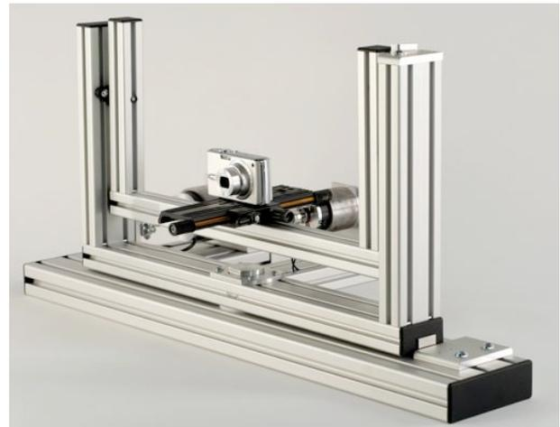
The device is delivered with camera mount and a controller box with a USB interface to the computer. To run the software provided with STEVE a Windows computer with a USB interface is required. A solid table or pedestal is useful.
