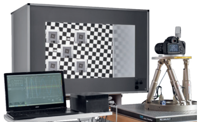
OIS test with the STEVE 6DL and the iQ-AF Box
