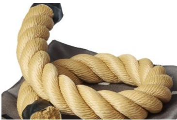
15 + 16) Sharpness and resolution, as well as low contrast detail, can be surveyed from the rope. Our rope consists of structures with different spatial frequencies.
