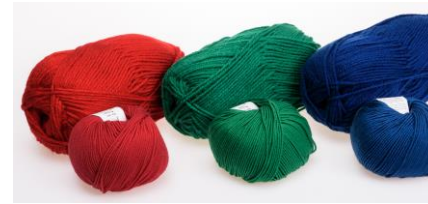
3) The red, green, and blue colored balls of wool are used to visualize the camera's ability to reproduce low contrast/fine detail in different colors.
