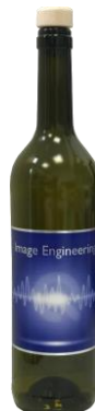
5) The wine bottle with fine details on the label is a challenge for the resolution of the camera. The sharpness and readability of the text is an important issue. In the dark areas the shadow details can be evaluated.
