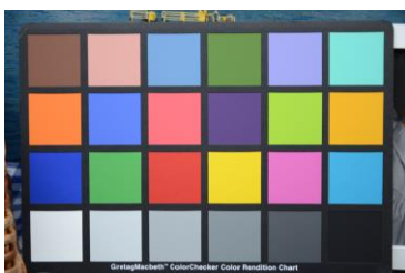
7) If there is a standard color chart in the world it is the X-Rite ColorChecker. This chart is used everywhere to check the color fidelity of cameras.
