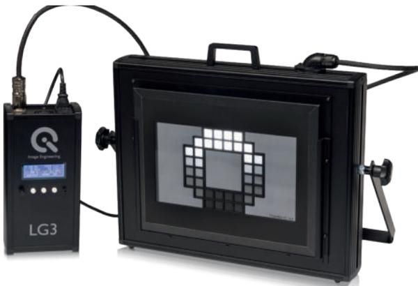
LG3 with OEFC test chart TE269C
