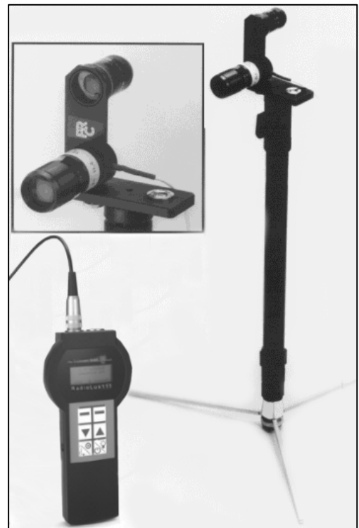
Fig. 5: Luminance measurement with luminance adapter and sighting telescope
