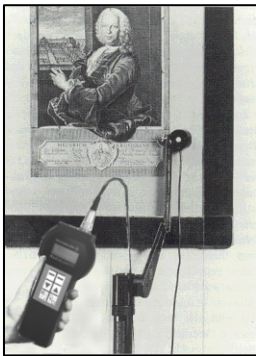
Fig. 4: Museum adapter with tripod for measurement at any inclined exhibits or space limiting areas
