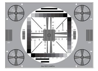
The TE95 test chart is designed for general (visual) appraisal of electronic cameras.
