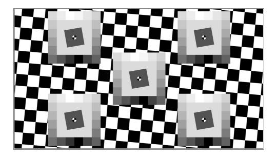
The TE261 Slanted Edges target has a tilted chequerboard in the background and 5 low contrast slanted edges together with surrounding gray patches in the front.
