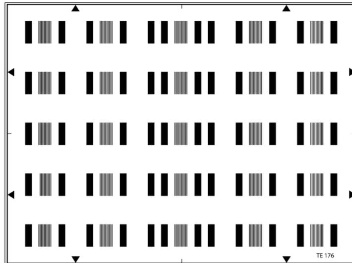
The test chart consists of alternating black and white bars with sharp transition (3-5 micrometers). The spatial variation of the density of these bars is a rectangular function of a cyclic ratio equal to 1. Two groups of bars with video frequencies of 0.5 and 5 MHz are distributed over the picture area whereby the 9 outer and middle positions each are essential for the measurements (the vertical, horizontal and diagonal axes, 10% within the extremities).
