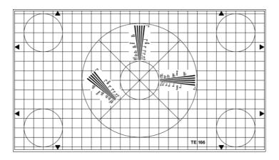
On a light background a grid structure of 25 horizontal and 15 vertical lines is arranged. The width of the grid lines is 0.13% of the picture width. The large circular line has a diameter of 82% of the picture height, the 5 small circular lines have a diameter of 27.4% of the picture hight. Inside the large circular line 3 resolution wedges are arranged at 0°, 90° and 135° corresponding to signal frequencies of 2-12 MHz (the markings end at 10 MHz resp. 800 TV lines).
