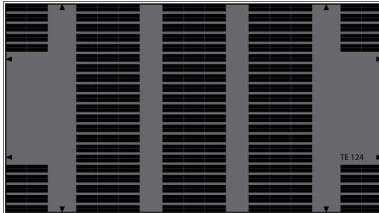
The test chart with an aspect ratio of 16:9 shows in the middle area 9 blocks containing 42 resolution patterns each. The corner fields have 20 resolution patterns.
