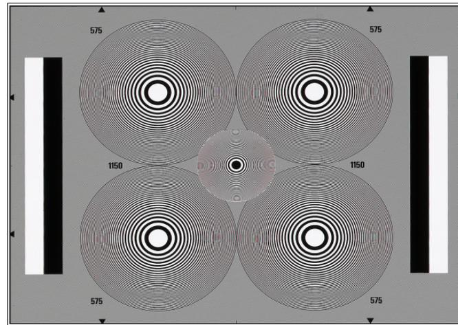
Checking resolution characteristics and cross color interferences of TV cameras and TV transmission systems
