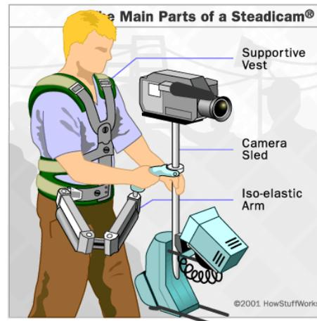
Figure 14: Main parts of SteadiCam [14]
