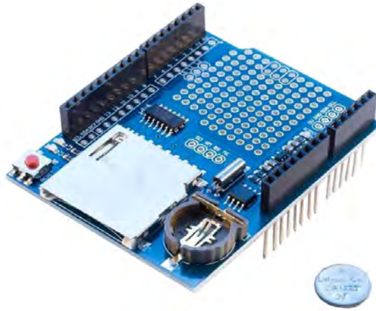
Figure 7 Data Logger Module [15]
