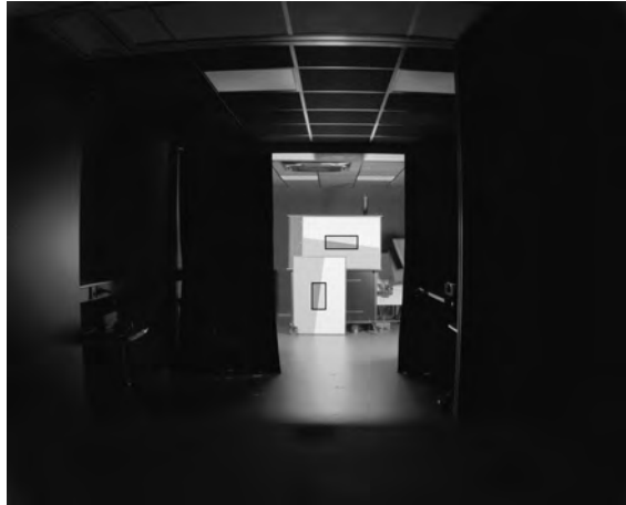
Figure 39 Example Check Image with marked ROI - IMX623
