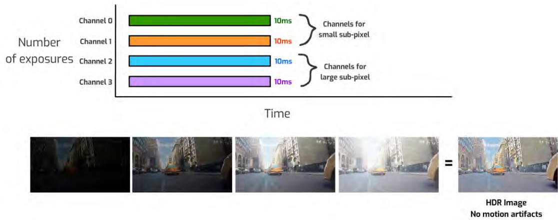
Figure 4 IMX490 Subpixel Channel [9]
