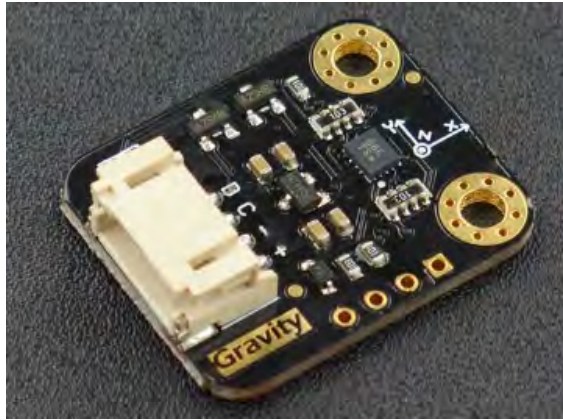
Figure 5 DFRobot I2C BMI160 6-Axis Inertial Motion Sensor [12]
