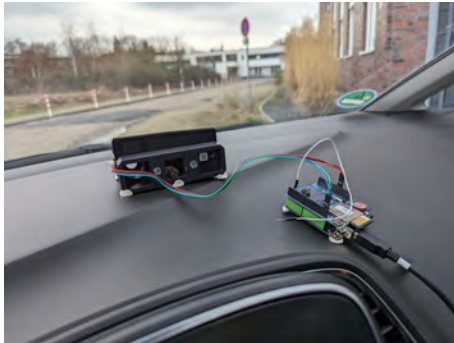
Figure 19 IMU Installation in Test Car
