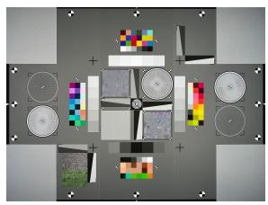
Figure 9. Target used for wide module evaluation.
