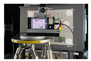
Figure 5. Setup for evaluation image stabilisation.
