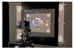
Figure 3. Setup for evaluation of selfie camera.
