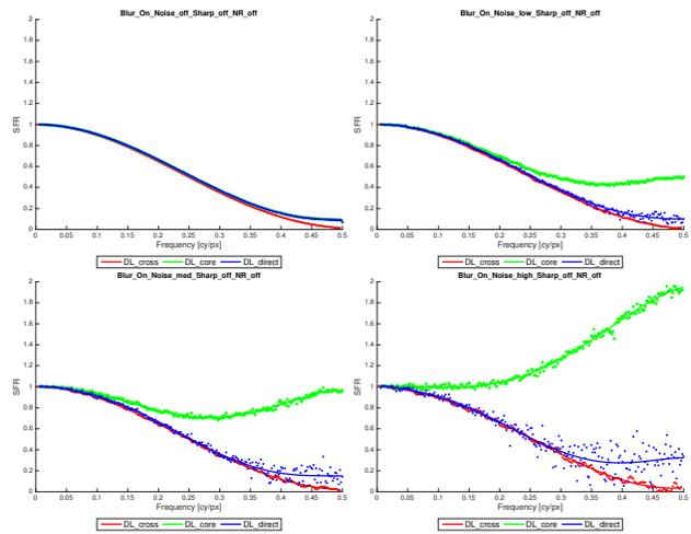
**Figure 6.** Simulation results; SFR based on the analysis of the same Dead Leaves pattern using three different analysis methods. Solid line: 3rd degree polynomial fit of obtained data (dots). **Top:** Blur filter applied, no noise added. **Others:** Blur filter applied, added white gaussian noise with a standard deviation of  $\sigma = 4, 8, 16$  (8 bit scale range)(low, medium, high)).
