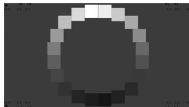
**Figure 3.** Test target used for noise measurement according to ISO15739:2013 (TE264)- the chart consists of 20 uniform gray patches.
