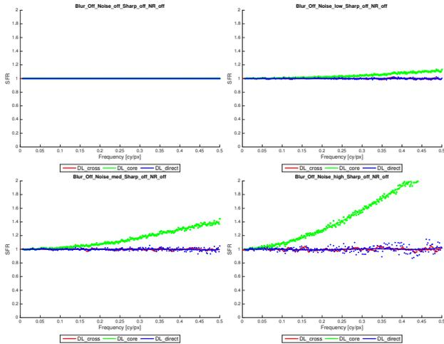
**Figure 5.** Simulation results; SFR based on the analysis of the same Dead Leaves pattern using three different analysis methods. Solid line: 3rd degree polynomial fit of obtained data (dots). **Top:** No noise added. **Others:** Added white gaussian noise with a standard deviation of  $\sigma = 4, 8, 16$  (8 bit scale range)(low, medium, high).
