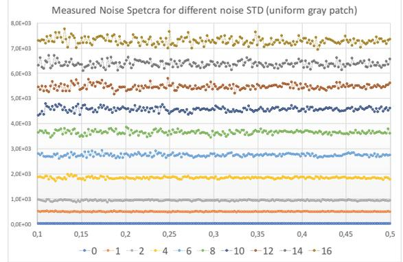
**Figure 9.** The measured Noise Power spectrum of the added noise. X-Axes show spatial frequencies in the range [0.1...0.5] The measured PS\_Noise on uniform gray patch
