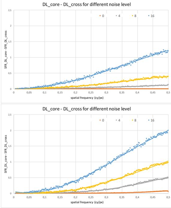
**Figure 8.** The difference between the SFR obtained from DL\_core and DL\_cross method for the four different noise level also used for the other simulations ( $\sigma = 0, 4, 8, 16$ ) Solid lines are polynomial trend lines. **Top:** No Blur Filter **Bottom:** Blur Filter applied
