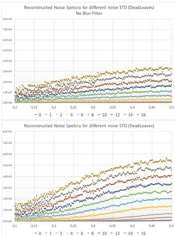
**Figure 10.** The reconstructed noise power spectrum. X-Axes show spatial frequencies in the range [0.1...0.5] Reconstructed Noise according to Equation 5 on DeadLeaves patch. **Top:** No Blur Filter **Bottom:** Blur Filter applied
