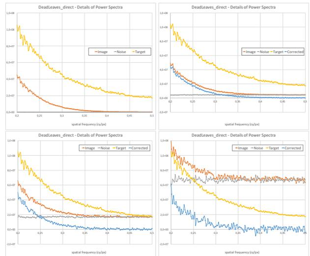
**Figure 7.** Direct comparison of different components that lead to the DeadLeaves.direct results as shown in Figure 6 Detail of the power spectra used to calculate the DeadLeaves.direct SFR (frequency range [0.2...0.5]). From top to bottom: No noise, low, medium and high noise. Corrected equals  $PS_{image} - PS_{Noise}$
