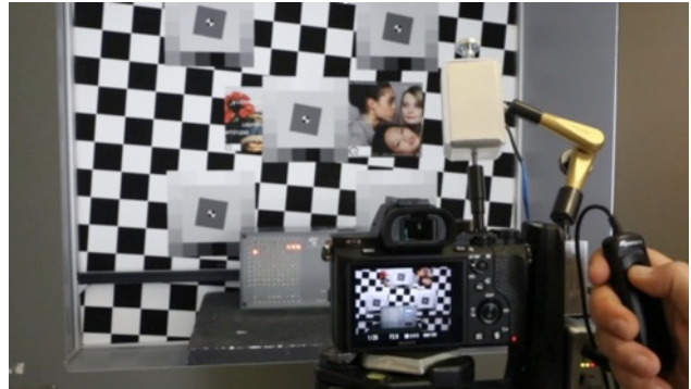
Figure 6. The AF speed measurement setup. A mechanical finger is synchronized with a timing device. As soon as the operator activates the process, the release button of the camera is pressed and the timing device starts at the same time. The delay between pressing the release button and capturing the image can be checked in the captured image.
