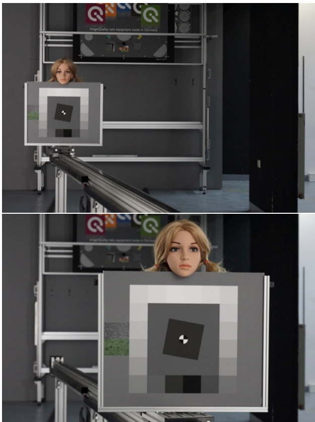
Figure 10. AF Tracking measurement setup. Example of captured images in minimum and maximum distance.
